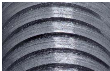
After tapping 184 holes with VUSP CH taps the surface finish is still excellent.
