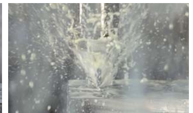
Discharge at pressure of 6 MPa (60 Bar)
