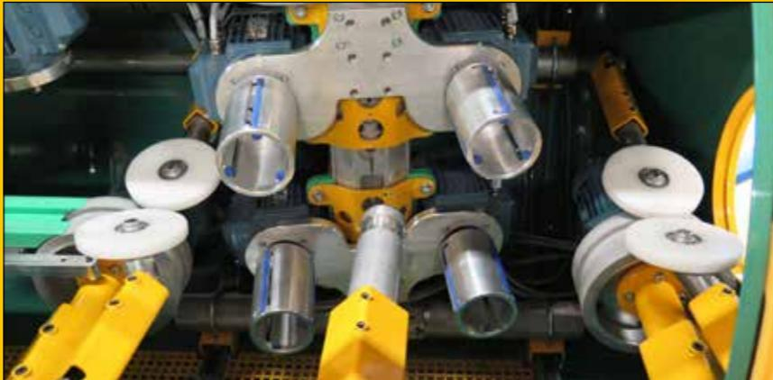
The tools being used are abrasive brushes in different size and density.
