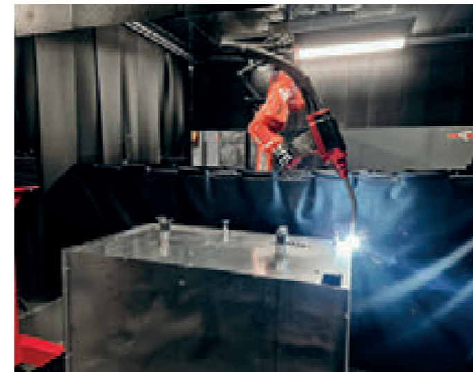
At Eurofours, Valk Welding installed a solution consisting of a Valk Welding FRAME-H concept, a TL-1800 robot, and an integrated power source with Panasonic’s Super Active Wire welding process.
