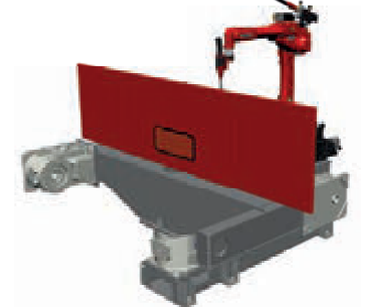
FRAME-IT+H with turning table and robot at the back side
