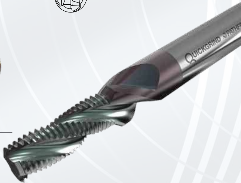
TM-IT tools are left handed – for CNC use M04 code
