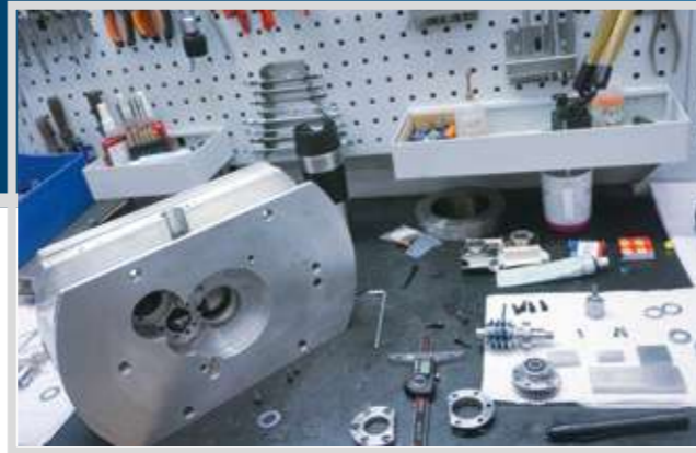
REPAIR WORKS ON A FACING HEAD.
