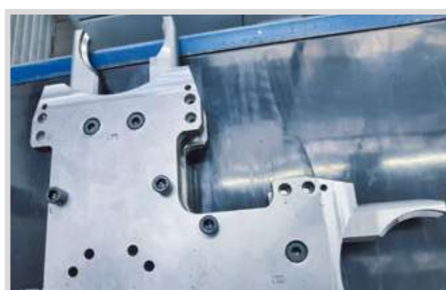
TOOL DOUBLE GRIPPER COMPLETELY ASSEMBLED.
