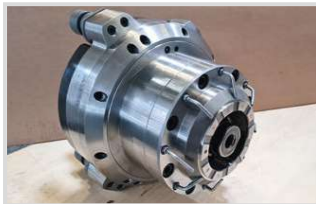
REPAIRED TURNING TOOL ADAPTER.
