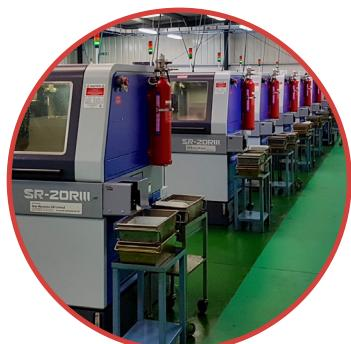
Should a high temperature or fire occur then the pressurised tubing will burst and the cylinder valve will activate deploying the extinguishant immediately onto the fire.
