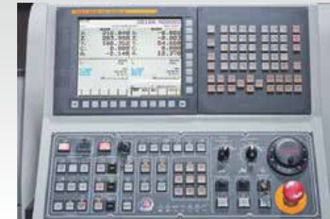
Fanuc 32i CNC Controller • Rotary control panel is easier for operator to use.
