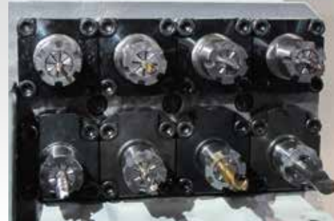
Sub-Spindle Tooling System with Y Axis • Apply to backside machining.
