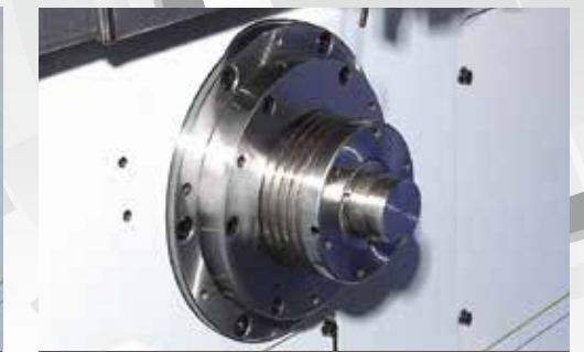
Non Guide Bushing Holder • For use in short parts and reduce rest bar.
