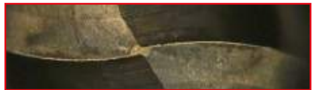
Edge condition (Flank wear)
