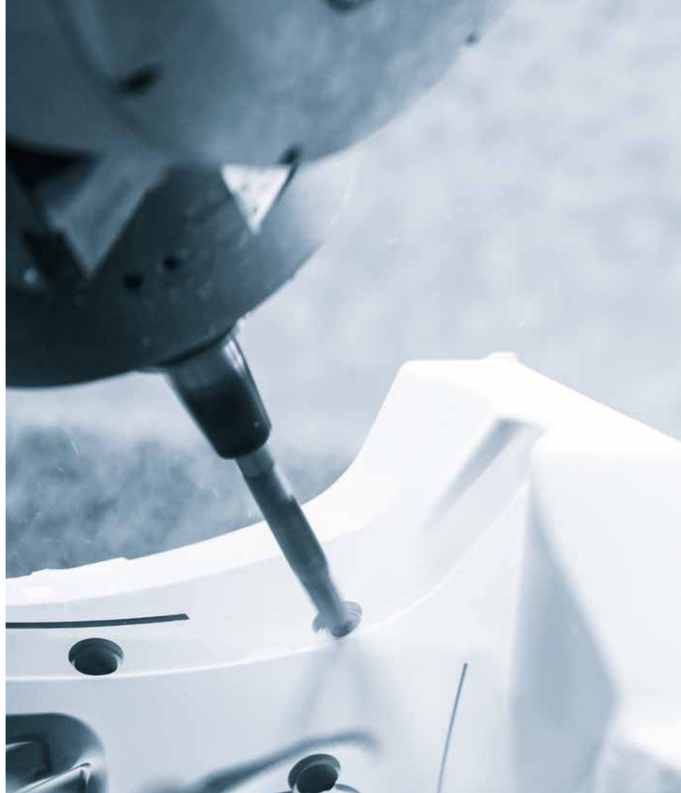
Clay models for design verification are generated in design model manufacturing and in design studios. For example, finished part models are processed using silicone molds to fabricate prototype parts for lighting systems.
