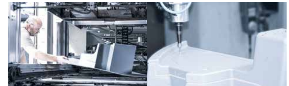
Thermoforming molds are needed for the series production of plastic parts. Tebis is often used here for trimming edges and cutouts.
