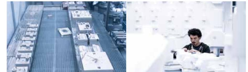
In foundry model manufacturing, Tebis customers produce all components, including models, mold boxes, sand molds and Exporit models needed for casting blanks in sheet metal die manufacturing.
