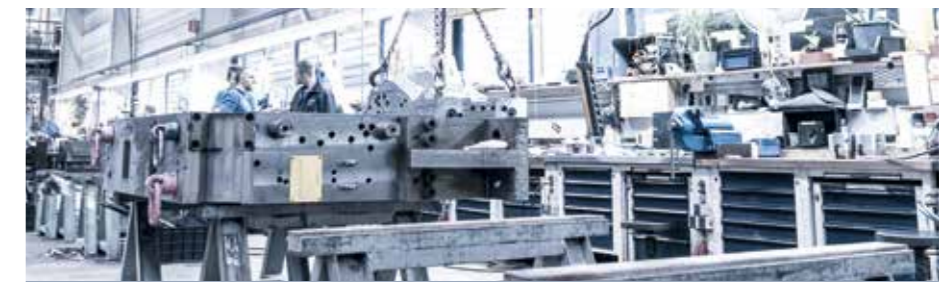
Die-casting molds and forging dies are used to manufacture metallic components, mostly for drive units.
