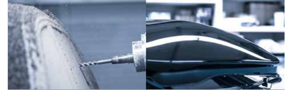
Clay models for design verification are generated in design model manufacturing and in design studios. For example, finished part models are processed using silicone molds to fabricate prototype parts for lighting systems.
