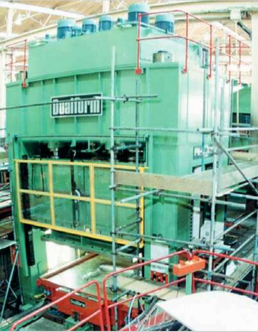
Main right: Top and bottom tools manufactured in the Dualform Model 9 press ready for pressing panels.
