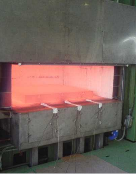
Main (right): 1400 tonne SPF/DB press complete with semi-automatic tool loading equipment
