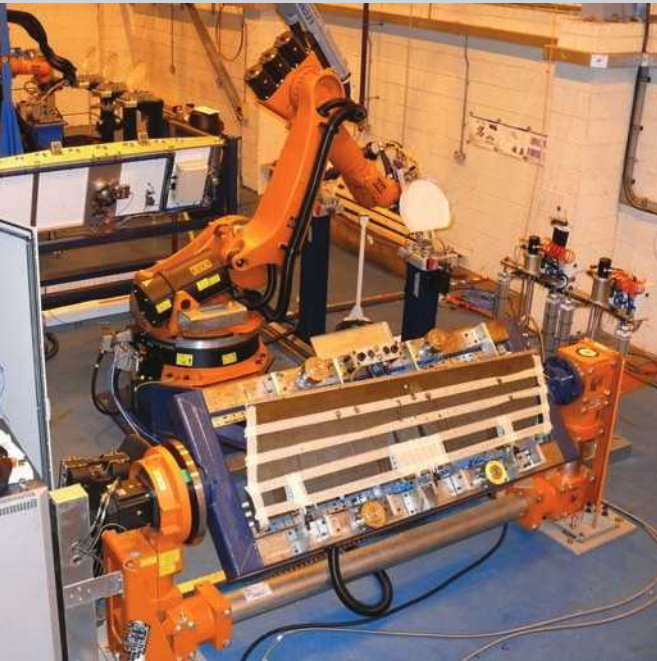
Left: Single step assembly robot for bonding aileron aircraft panels
