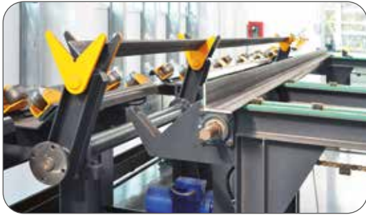
A stock length material transfer table with rotary loader can automatically index and load the next stock length as required.
