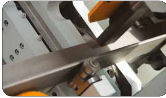
A CNC marking press can be provided to generate the required part number without any character set up.
