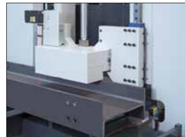
Laser measuring systems and a firm clamping device
