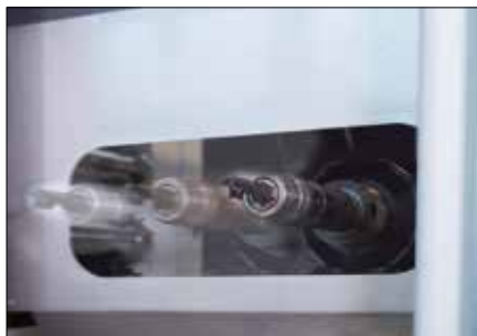
The auxiliary axis allows milling and scribing operations, as well a group of holes, thanks to its extra stroke.
