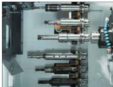
Automatic tool changer with 6 positions
