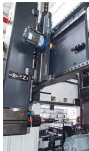
Auxiliary axes with 300 mm stroke
