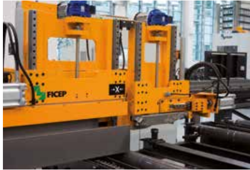
Second pincher for reduced overall dimensions
