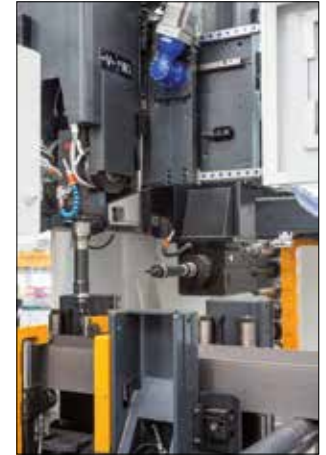
Second drill head with automatic tool changer
