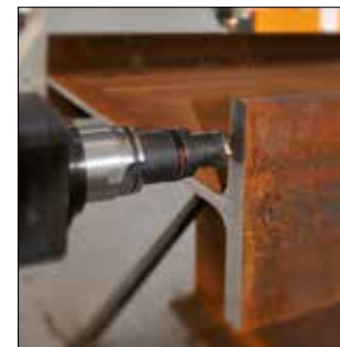
Mitering head for edge milling
