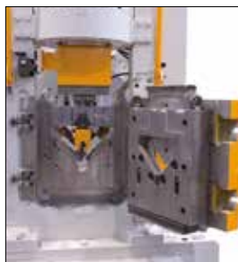
Quick change shear tooling for flats and channels
