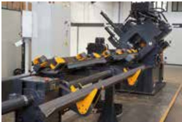
Rotating loading system to transfer the profiles onto the infeed table
