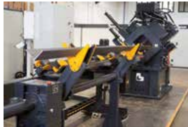
Rotating loading system to transfer the profiles onto the infeed table
