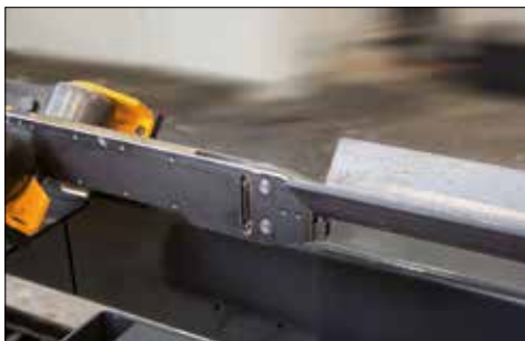
Pincher for precise material clamping
