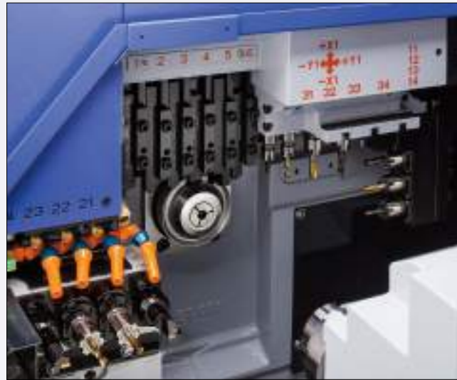
Photo: type G / (Cartridge type 5-spindle cross drilling unit)/N.G.B.type
