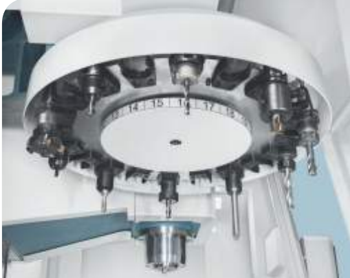
Automatic Tool Changer with 20 tools capacity (ROMI D 600)
